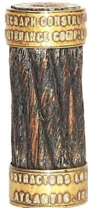
Figure 1: A small part of the 1,852 nautical mile Atlantic cable, laid in 1865.
